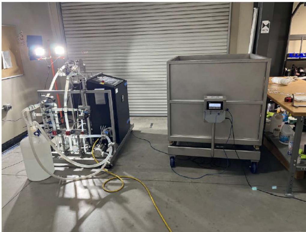
6-inlet 1" single-use ILD skid capable of diluting up to 40 LPM at a 1:10 ratio, with automatic pH and conductivity control; paired with the 1000L WFI tote.
